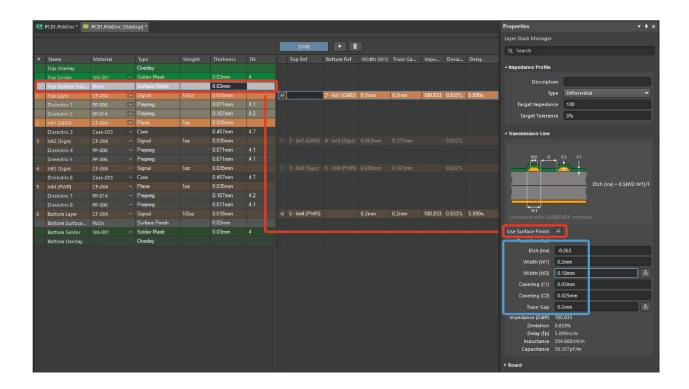
12. Select another material for the outer layer copper library by ½ oz (Thickness = 0.018mm). Since the copper thickness affects the impedance, and total thickness of the outer layers of the metal layer will be added to the copper plus the surface finish, it is possible to change the copper thickness to adapt the calculation to a given impedance. If such a material is available from the fabricator.
