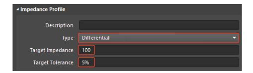
6. Select the layer where the transmission line will be located. Specify 1 layer (Top Layer) in the impedance profile, to high-light all layers in the stack-up that participate in the calculation of this transmission line (display the structure and parameters of this line). In the impedance profile in the Bottom Ref column - select the nearest reference layer 2 - Int1 (GND).
