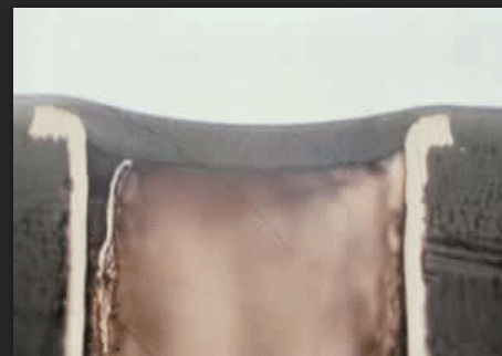
Inadequate size or number of vias
