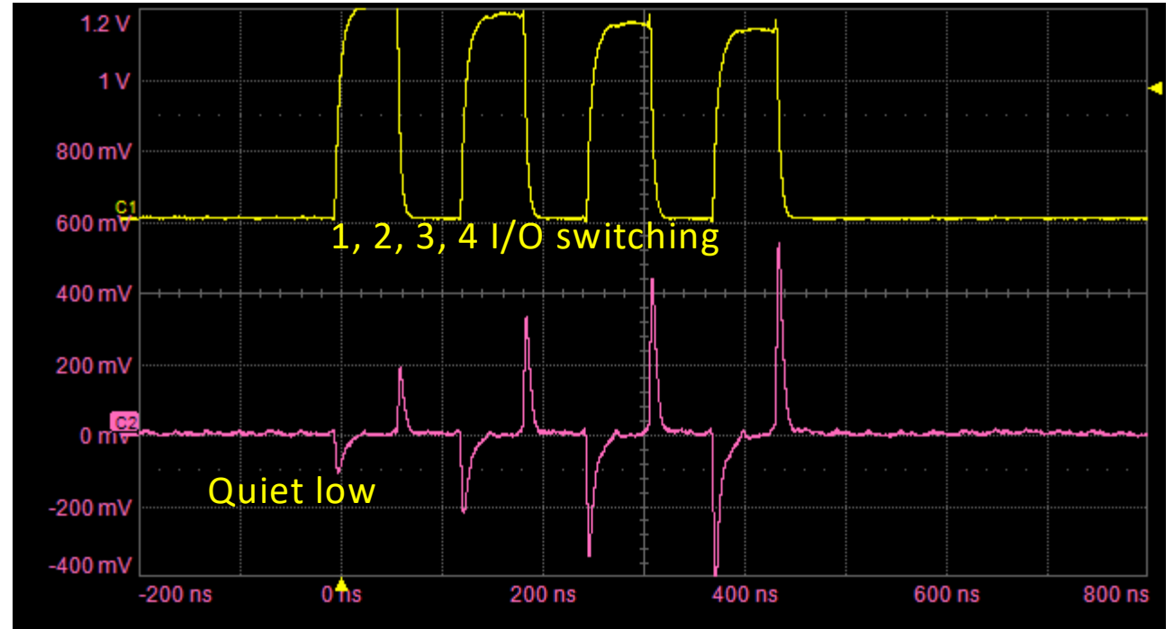
Ground Bounce Scales with the Number of I/O Simultaneously Switching and Sharing the Same Return Path
