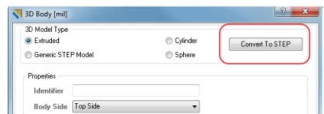
Figure 10: Next, convert the extruded shape into a STEP model.
