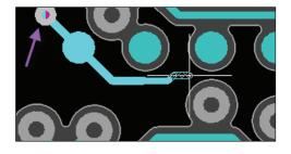
**Smaller Width** - There are options to use a width of any pre-defined proper width or any width you would like. Here the trace has been changed to a smaller width, and you can see the clearance web is gone, which means there is room to route through that gap.
