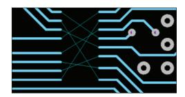
**Initial Routing** - Route out from both ends of the connection.
