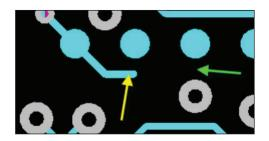
**Starting Point** - In the image below, you can see when routing the trace (yellow arrow) it seems that it would fit between the pad and via (green arrow).
