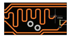
**Tune with Arcs** - You can control the radius of the arc or even have a semi-circle pattern. This image shows an arc replacing the 45-degree miter corner.
