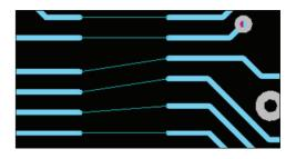
**Final Result** - Here is the outcome of the subnet swapping. Just route the traces together and you have optimized the exits from the BGA, making the overall routing task much easier
