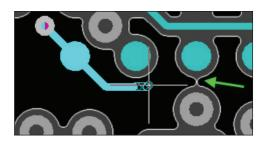
**Start Routing** - When the routing starts, the dynamic clearance boundary is shown, and you can see the web that is created (green arrow) which displays the trace will not fit. Whenever there is a web (large or small), it simply means the current trace will not fit through the gap.
