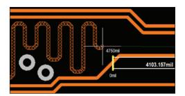
**Adding Tuning** - This tuning is being added with 45-degree miter corners. The Length Gauge shows that the target length is 4750 mil, and the current length is 4103.157 mil.
