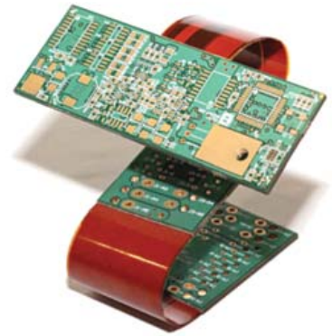
Figure 2: Typically, rigid-flex has the components mounted to rigid boards interconnected by flex circuits. The flex circuits let the assembly bend to fit the assembly into the product enclosure.
